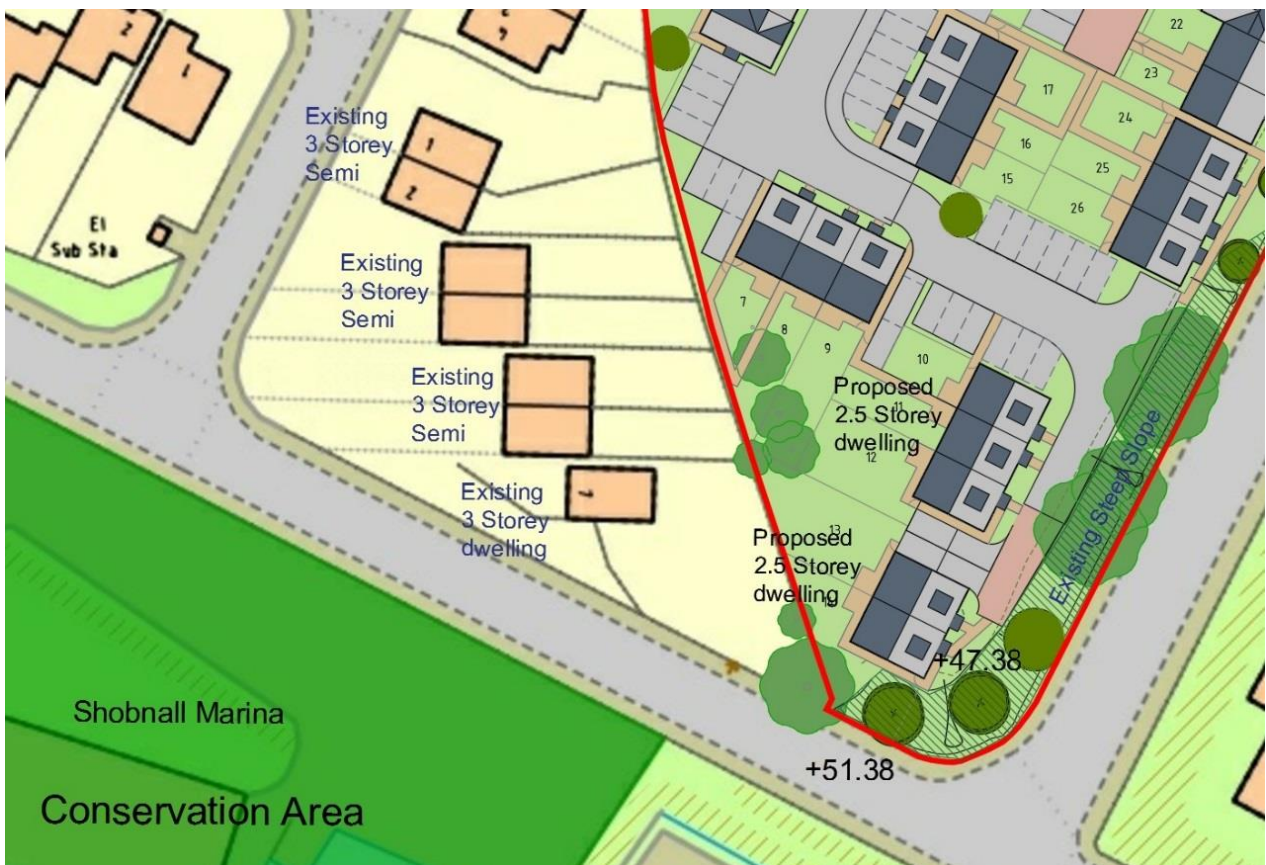
Illustration showing level difference between Shobnall Road, existing dwellings and proposed scheme.
